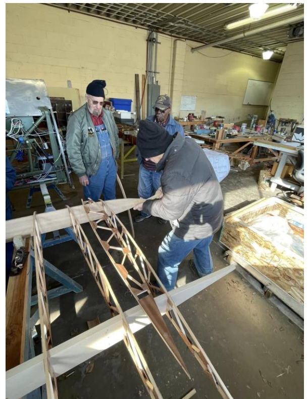
Howard Webb, Wat Watkins, Bob Szabados, working on Wing building -- cut, sand, fit, glue... repeat.
