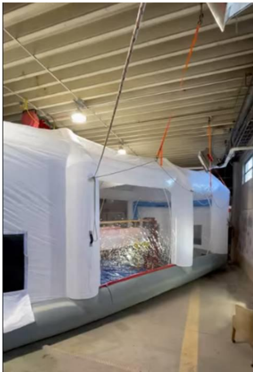
Portable Paint booth, outside view
