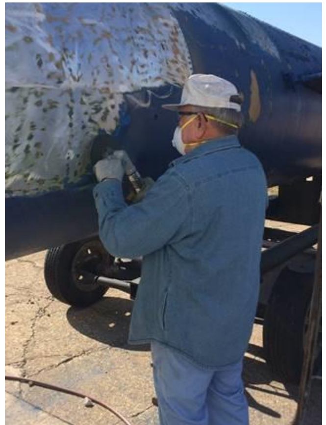
Earl Hastings grinding paint off the Regulus I cruise missile, March 14, 2019. Earl did a lot of sanding on the Regulus I cruise missile -- he would have a blue face around his paint mask from all the blue paint dust.
